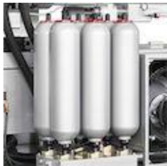
Accumulators on all the working phases of the machine
