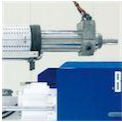
quick replacement of plasticization unit
